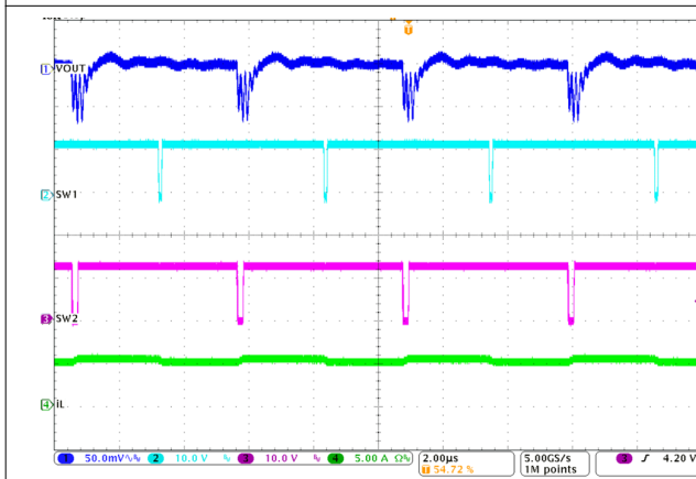
Figure 8-4. Switching Waveforms in V_{IN} = 12\text{ V} , V_{OUT} = 12\text{ V} , I_O = 5\text{ A} , FPWM
