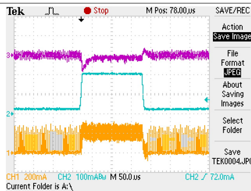
Figure 13. PFM Load Transient
