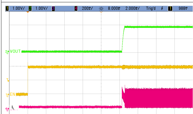
Figure 9-16. Startup Into 100 mA Electronic Load EN Delay + Soft-Start Delay
