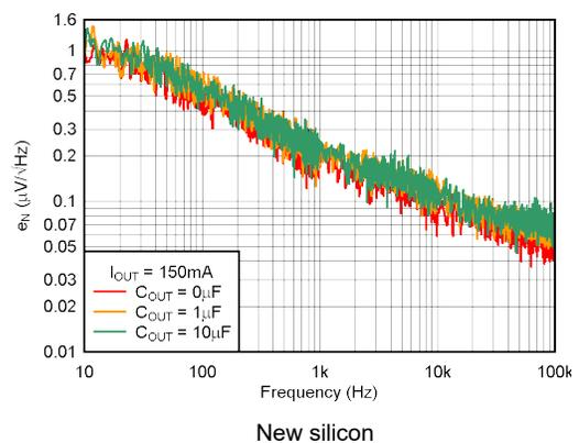
Figure 5-30. Noise Spectral Density  $C_{NR} = 0.01\text{ }\mu\text{F}$
