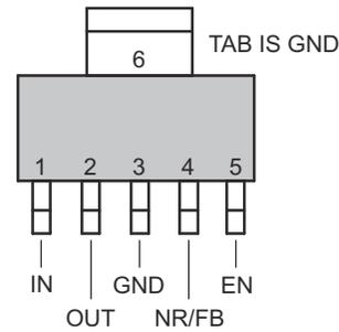
Figure 4-2. DCQ Package, 6-Pin SOT-223 (Top View)
