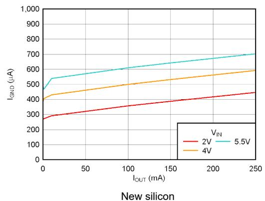
Figure 5-12. Ground Pin Current vs Output Current
