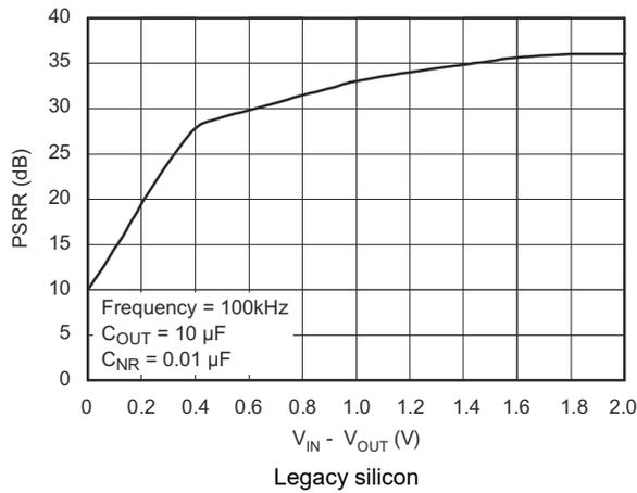
Figure 5-25. PSRR (Ripple Rejection) vs  $V_{IN} - V_{OUT}$
