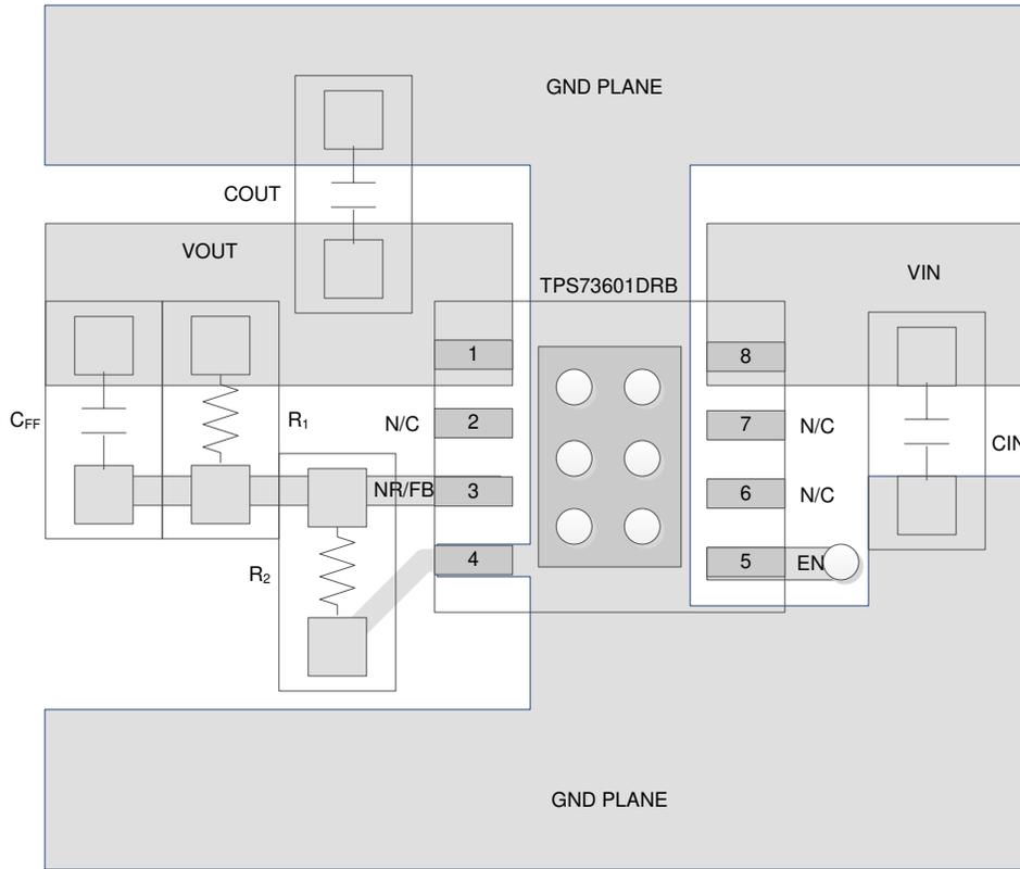
**Figure 7-9. Adjustable Output Voltage Option Layout (DRB Package)**
