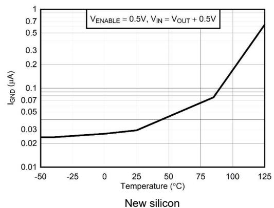
Figure 5-18. Ground Pin Current in Shutdown vs Temperature
