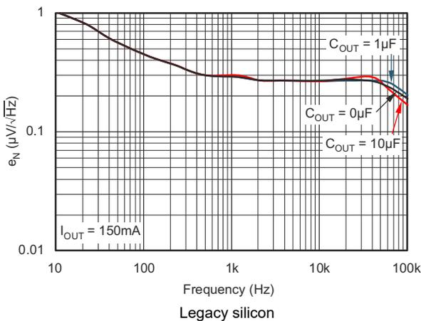
Figure 5-27. Noise Spectral Density vs  $C_{NR} = 0\text{ }\mu\text{F}$
