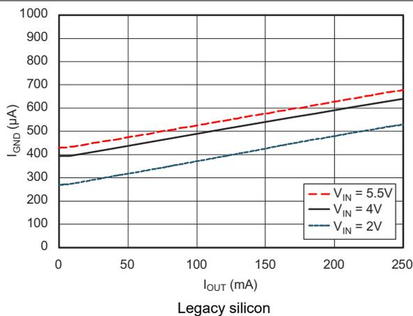
Figure 5-11. Ground Pin Current vs Output Current
