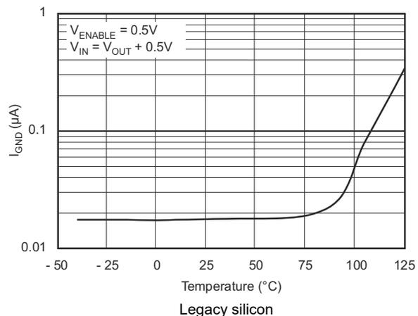
Figure 5-17. Ground Pin Current in Shutdown vs Temperature
