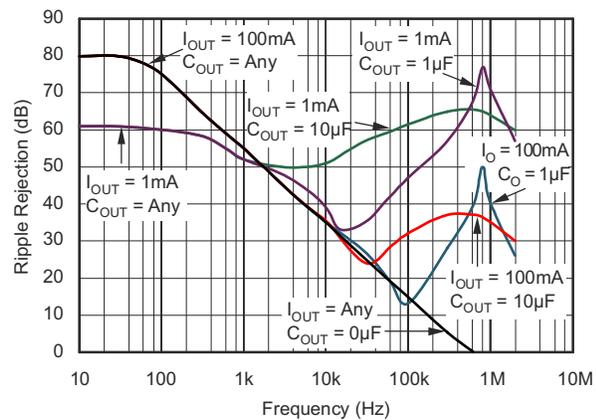
Figure 5-23. PSRR (Ripple Rejection) vs Frequency
