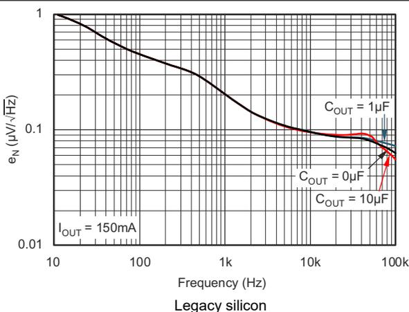
Figure 5-29. Noise Spectral Density vs  $C_{NR} = 0.01\text{ }\mu\text{F}$
