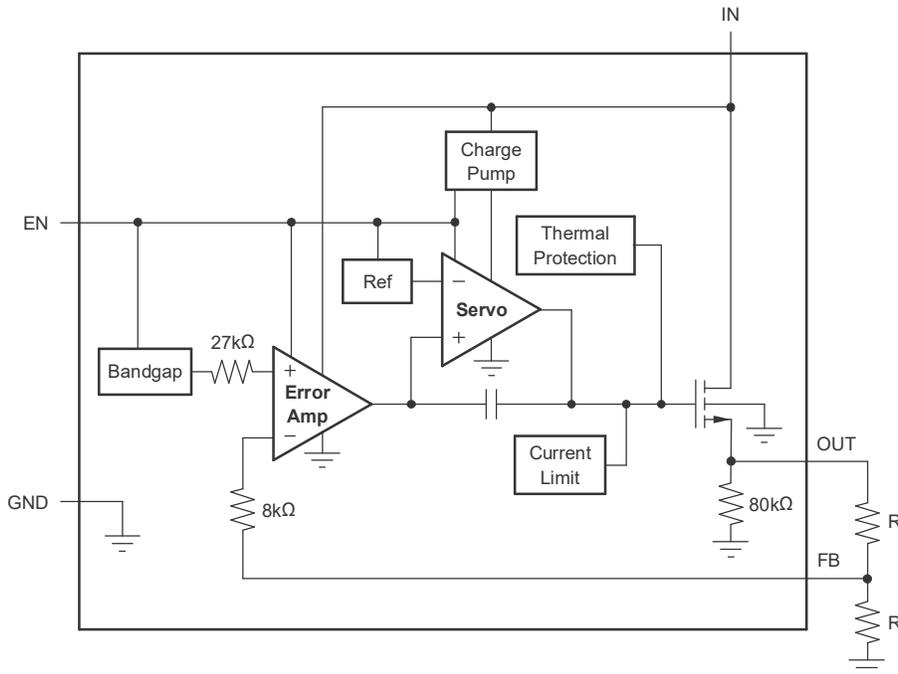
$$V_{OUT} = (R_1 + R_2) / R_2 \times 1.204$$
