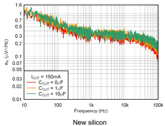
Figure 5-28. Noise Spectral Density  $C_{NR} = 0\text{ }\mu\text{F}$
