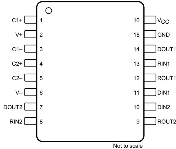
**Figure 4-1. D, DW, N or PW Package, 16-Pin SOIC or TSSOP
