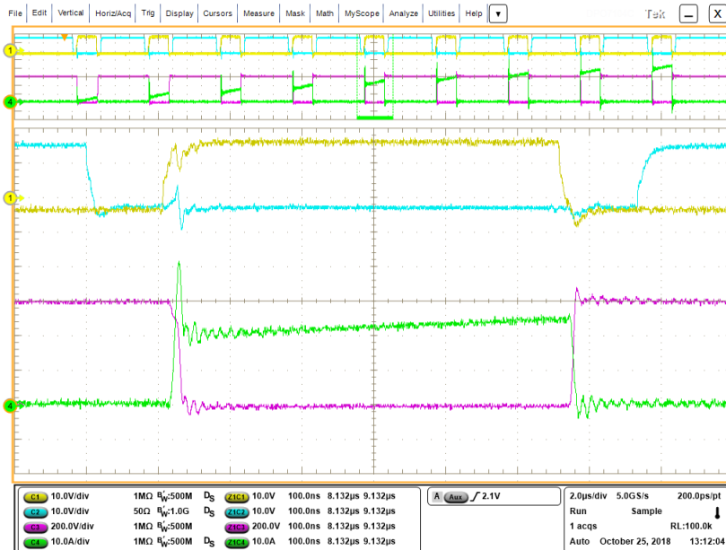
Figure 8-6. SiC MOSFET Switching Waveforms
