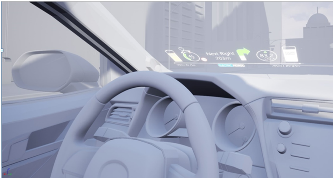
Figure 1-1. Digital windshield cluster (image courtesy of Ceres Holographics)
