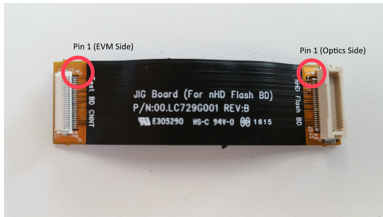
Figure 2. 0.2 nHD Optical Engine Flex Cable Connector Overview
