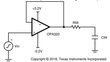
2. Select the components for the adjustable LDO outputs. Using the previous OPA320 example, the rails for the system are –200mV and +5.2V.
