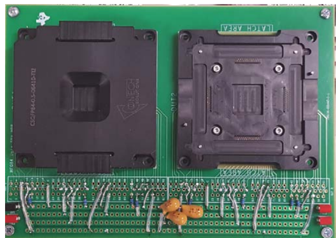
Figure 3. ADS1278 84-HFQ Diagram and Bias Board
