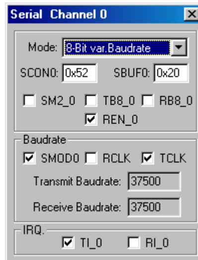
Figure 17–18. Serial Channel 0 Communication Peripheral
