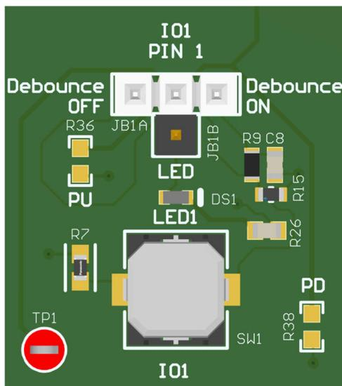
Figure 2-3. Switch/LED Blocks
