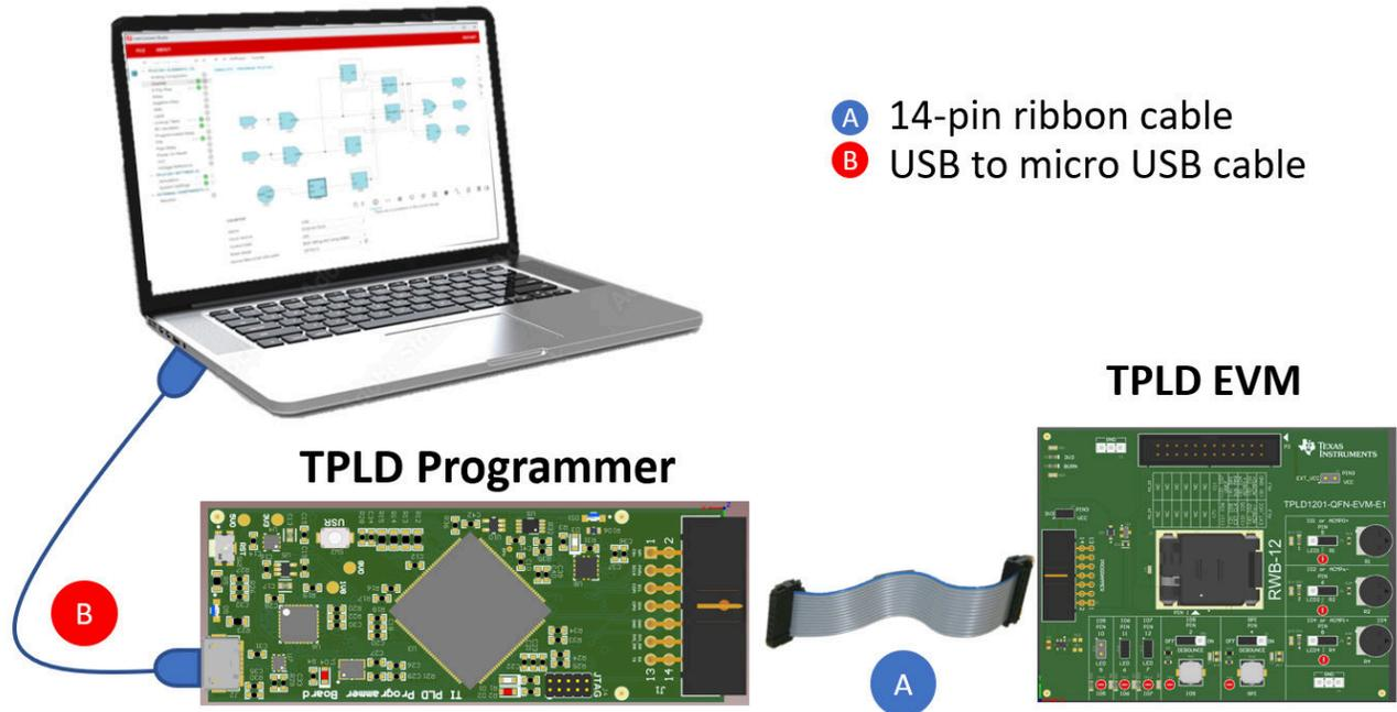
Figure 3-1. Connecting a TPLD EVM and Programmer
