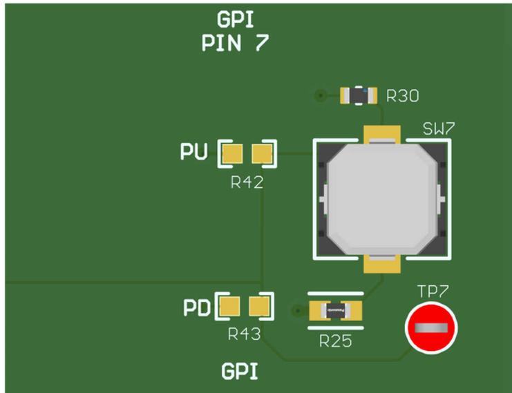
Figure 2-4. GPI Switch Block
