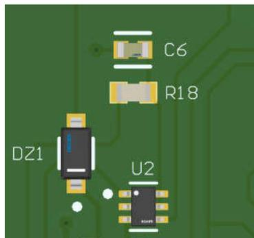
Figure 2-2. GPI Protection Block
