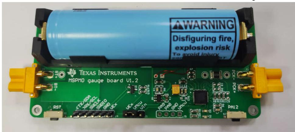
**Figure 1-1. MSPM0 Gauge Hardware Board**
