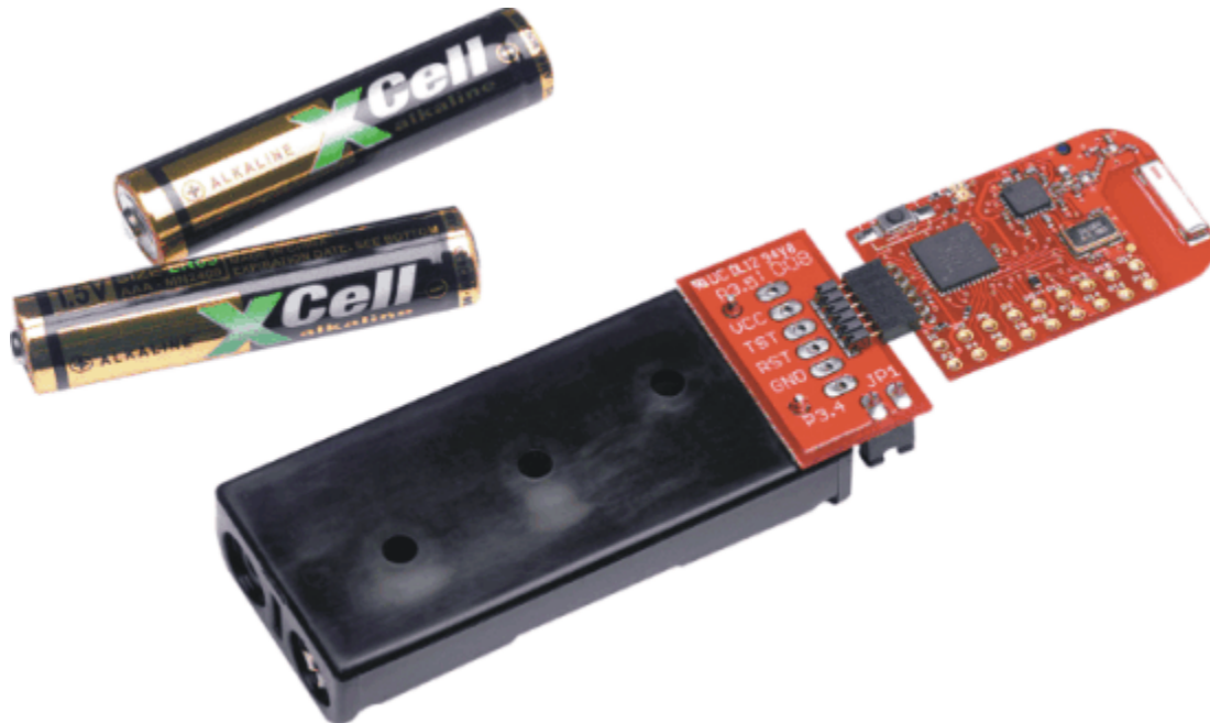
Figure 2. eZ430-RF2500 Battery Board
