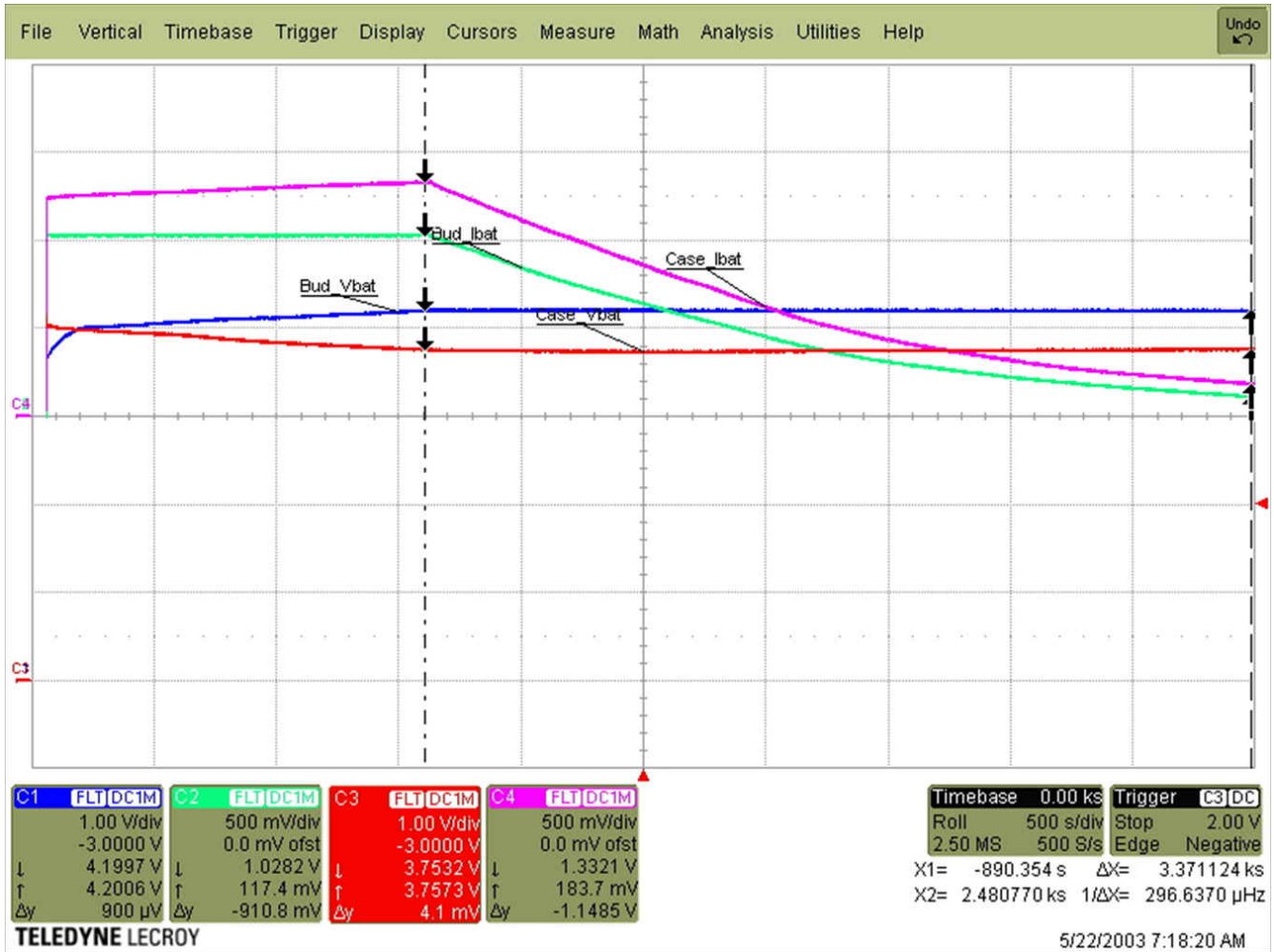
Figure 6-3. Charge Cycle of the BQ25619 with 4.6-V Output Design
