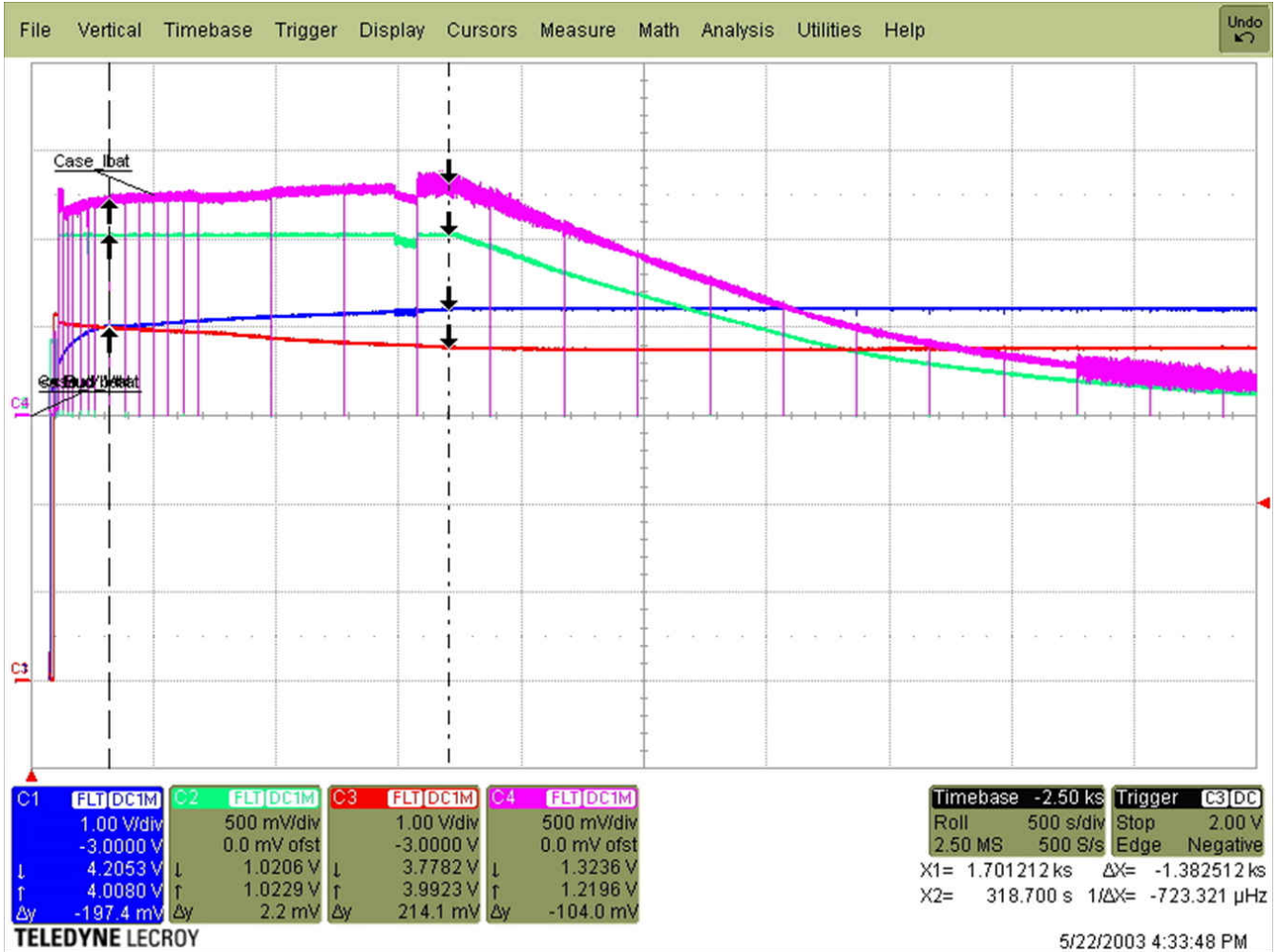
Figure 6-1. Charge Cycle of the Dynamic Voltage Adjustment Design
