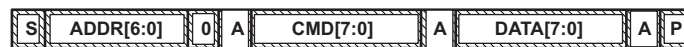
Figure 2-9. Attempt to Write a Read-Only Address (Nack After Data Sent By Master)
