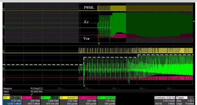
Figure 14. Recovery after OPP with 3 Stages of Peak Current (CH1 = PWML, CH4 = Transformer Primary Winding Current, CH2 = Switch Node Voltage)
