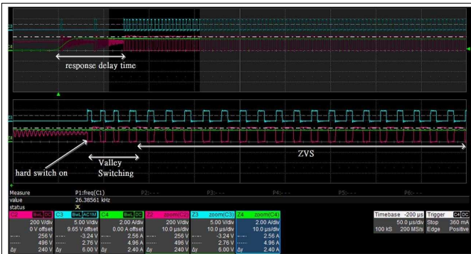
Figure 31. Load Transient Step-Up (0A to 2.25A)
