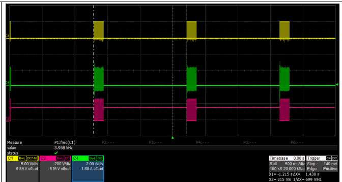
Figure 28. OPP Auto Retry (CH1 = PWML, CH2 = Switch Node Voltage, CH3 = Transformer Primary Current)
