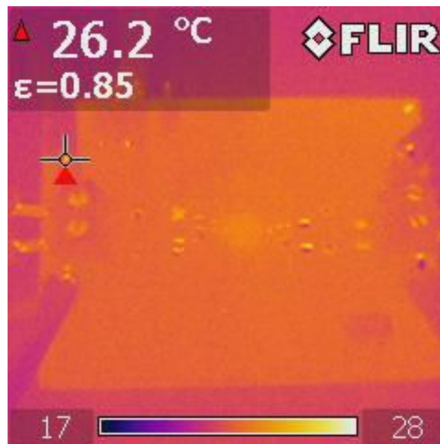
Figure 3-29. UCC33020-Q1 VINP=3.3V, VCC=5.0V, Iout=0mA, Pout=0W, TA=25°C
