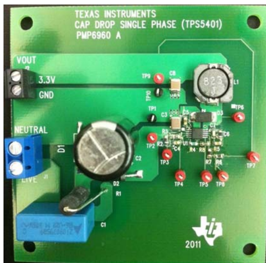
Figure 1. Single Phase Cap Drop E-Meter Design (PMP6960) using the TPS5401
