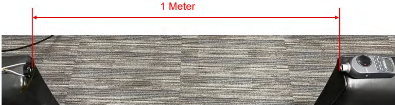
Figure 3-1. SPL Test Setup Performed with Radio Shack SPL Meter
