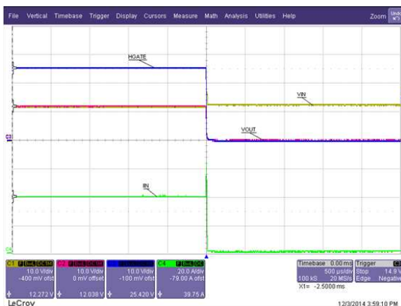
Figure 7. Hot Short on V_{OUT} (Zoomed Out)
