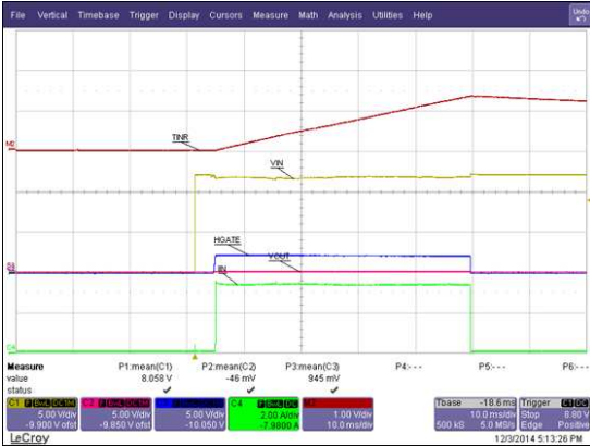
Figure 11. Start into Short on VOUT
