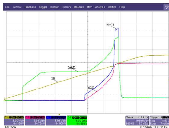
Figure 9. Under/Overvoltage With V_{IN} Rising
