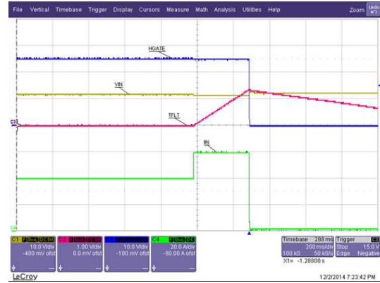
Figure 12. Load Step – 40 A to 60 A
