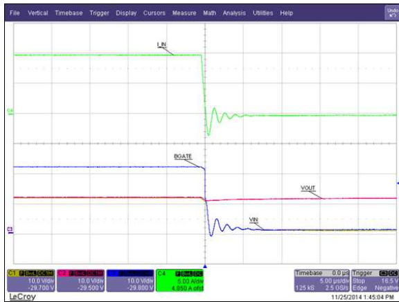
Figure 13. Hot – Short on VIN
