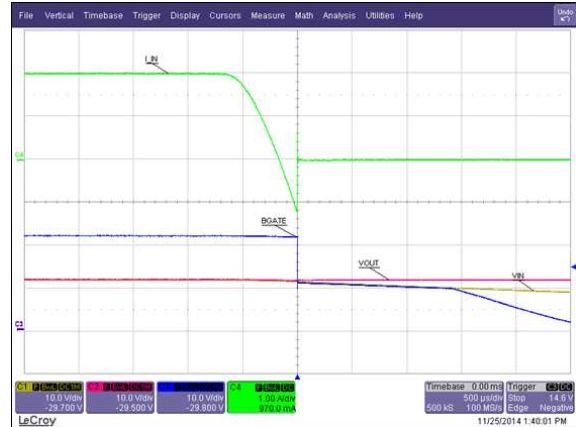
Figure 14. Gradual Reverse Current
