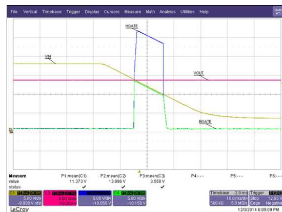
Figure 10. Under/Overvoltage With V_{IN} Falling
