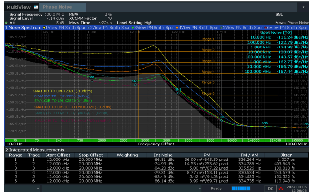
Figure 5-12. Total RMS Jitter (10Hz - 50MHz): 10MHz Reference Input to LMX2820 100MHz Output With or Without Buffer (Case 1: T1 to T3, Case 2: T4 to T6, Input power: -10dBm, 0dBm, 14dBm)
