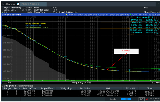
Figure 6-7. RMS Jitter (12kHz - 1MHz): 10MHz Output - LMK1C110x vs Competition
