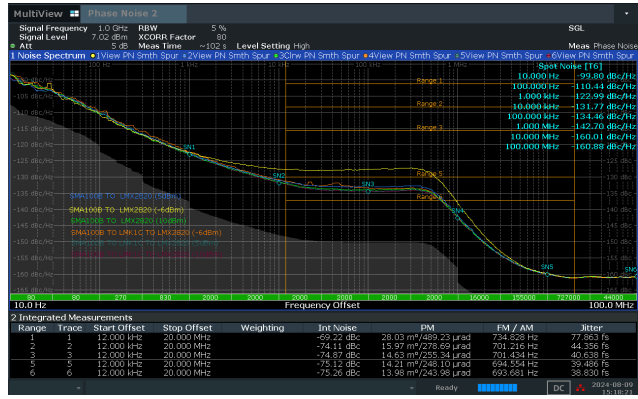
Figure 5-10. Total RMS Jitter (12kHz - 20MHz): 10MHz Reference Input to LMX2820 1GHz Output With or Without Buffer (Case 1: T1 to T3, Case 2: T4 to T6, Input power: -6dBm, 5dBm, 10dBm)
