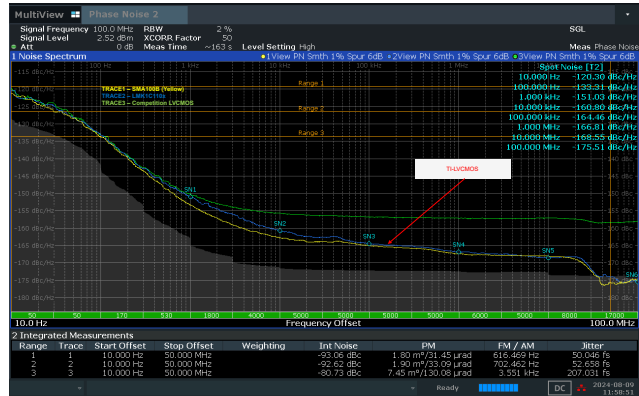
Figure 6-10. RMS Jitter (10Hz - 50MHz): 100MHz Output - LMK1C110x vs Competition
