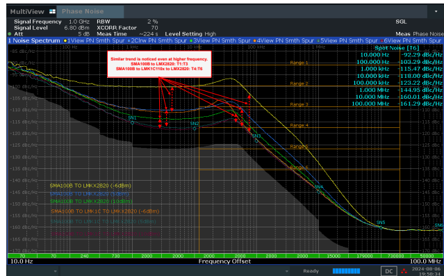
Figure 5-6. 10MHz Reference Input to LMX2820 1GHz Output With or Without Buffer (Case 1: T1 to T3, Case 2: T4 to T6, Input power: -6dBm, 5dBm, 10dBm)
