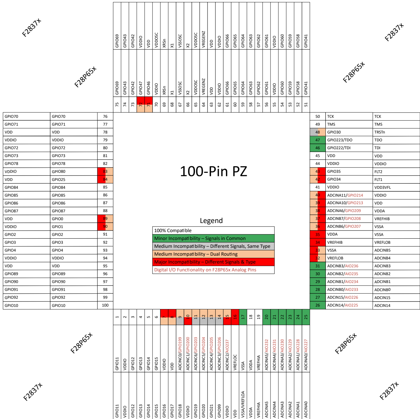
Figure 2-2. F2837x and F28P65x 100-Pin Overlay
