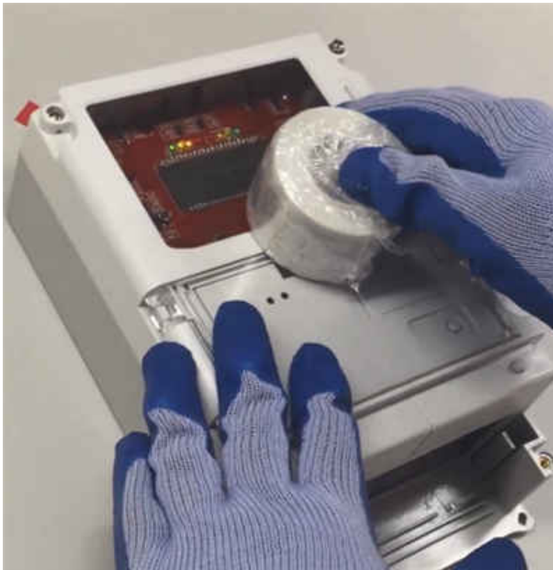
Figure 1. The magnetic tamper detection reference design with an external tamper magnet
