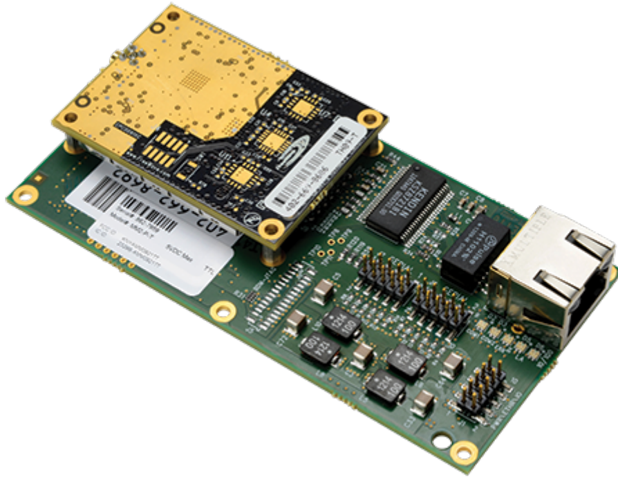
Figure 2. Non-enclosed, board-level version of the ZumLink Z9-PC IPR
