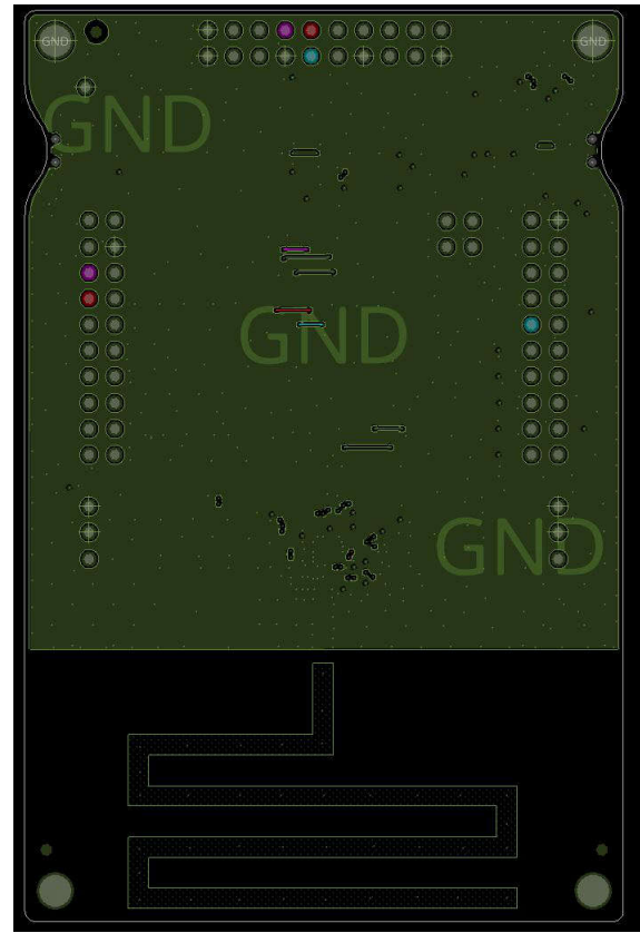
Figure 3-4. Bottom Layer of the 4-Layer PCB Design
