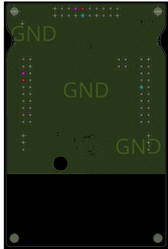
Figure 3-2. Second Layer of the 4-Layer PCB Design
