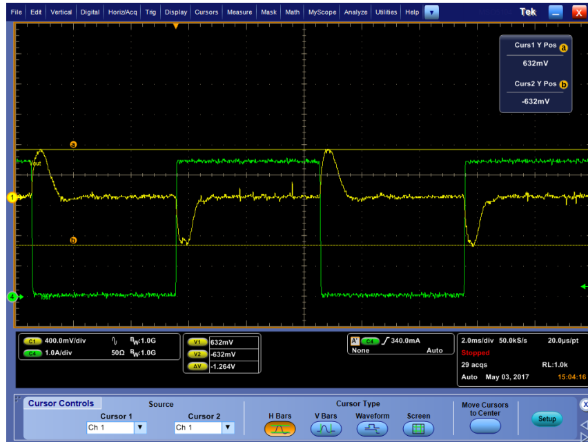
Figure 2-13: V_{out} = 52V , I_{load} = 0.1A-4.5A-0.1A . V_{pp} = 1.26V , V_{in} = 48V
