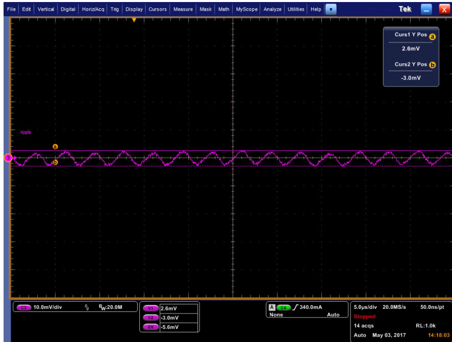
Figure 2-5 Vout =28V, Vin =36V, Iout = 0A. Vpp = 5.6mV
