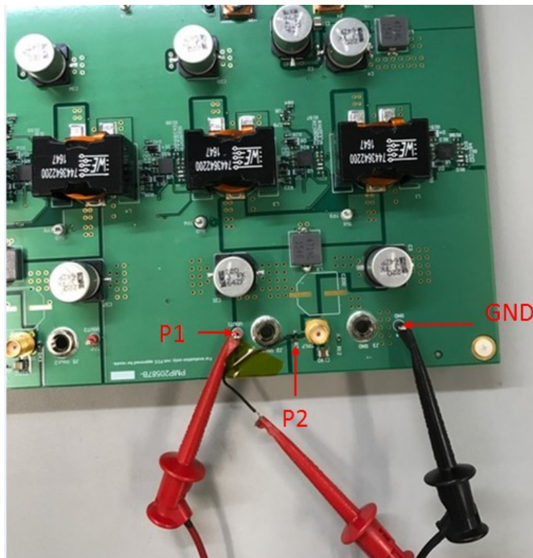
Figure 2-19 Bode Plot Measurement Setup
