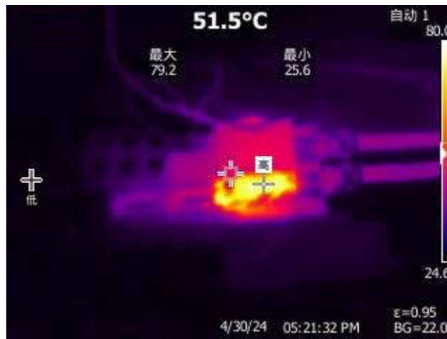
Figure 2-4. Thermal Image 8V IN , With 1.4A Load
