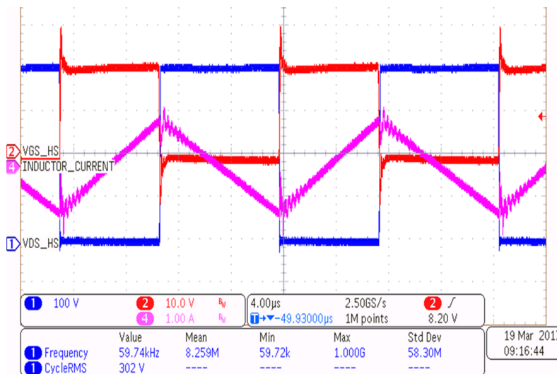
Figure 25. High-Side Switching Waveform
