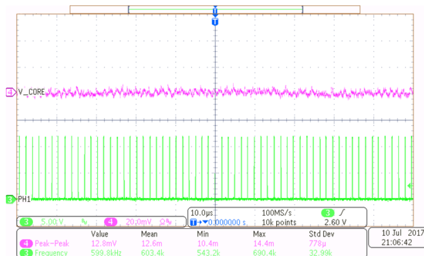
Figure 7. Core Rail — Steady State, 200 A
