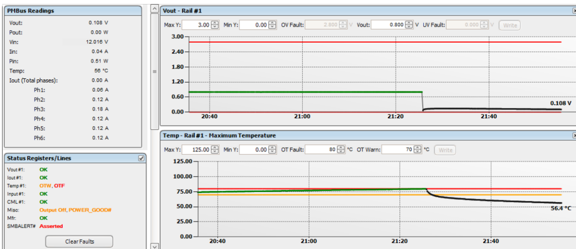
Figure 30. Overtemperature Shutdown as Seen in Fusion GUI
