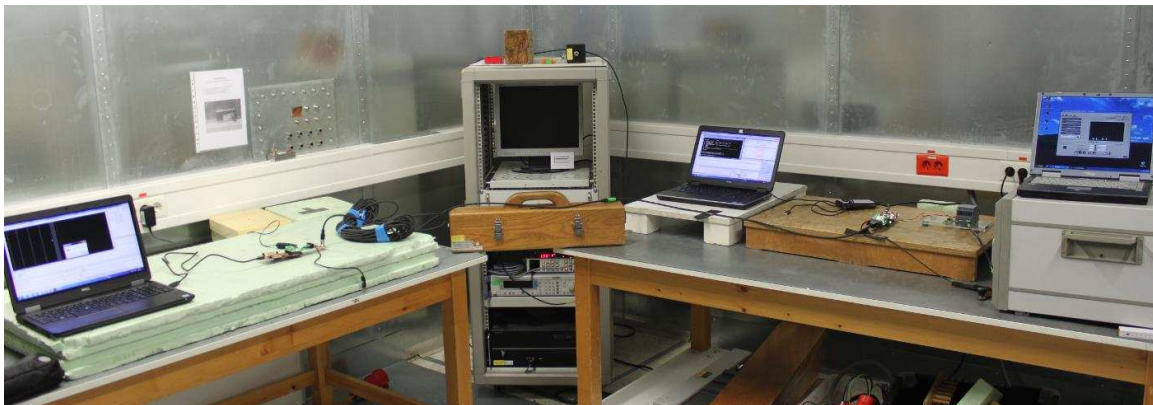
Figure 21. Picture of Test Setup for EMC Immunity Tests Using Same Transceiver and Direct EFT Connection
