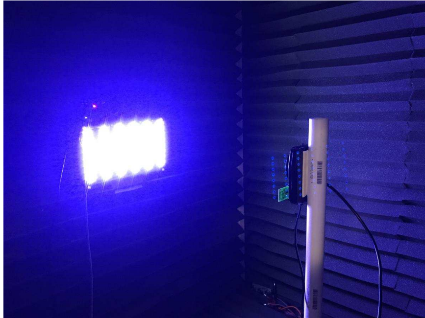
Figure 30. TIDA-01008 Illuminance Sensing Testing
