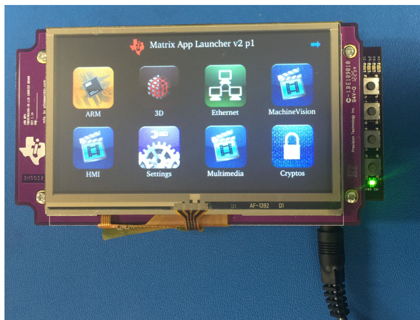
Figure 5. AM335x Starter Kit Setup (LCD Face Up)
