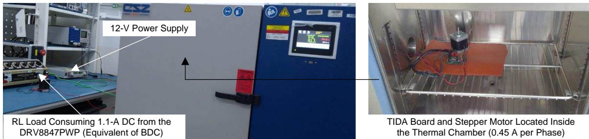
Figure 45. Setup for Testing the Design at Multiple Ambient Temperatures
