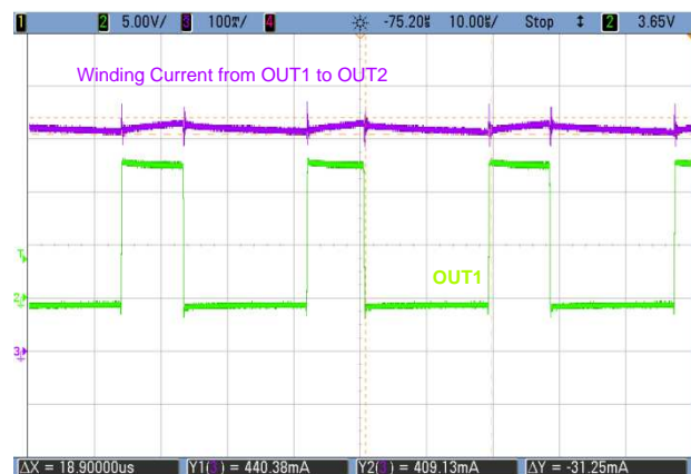
Figure 28. Current Regulation With Slow Decay Mode
