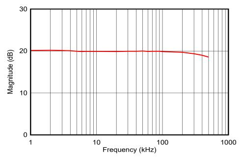
Figure 3-3. Transfer Curve of Gain Stage
