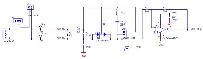
Figure 2-2. Schematics Current Sensing Circuit
