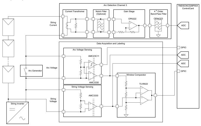
Figure 3-8. Test Setup for Test With Real Arcs
