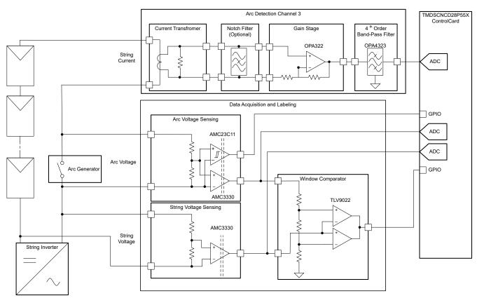
Figure 2-5. Block Diagram Arc Test Setup
