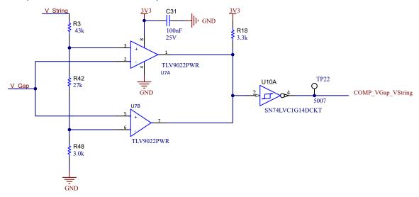
Figure 2-9. Schematics Window Comparator Circuit for Arc Labeling
