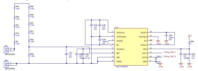
Figure 2-6. Schematics String Voltage Sensing
