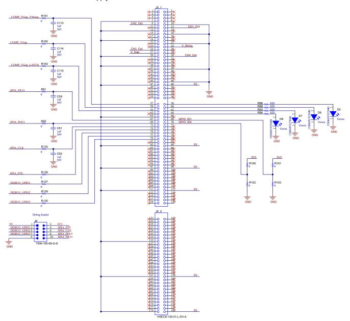
Figure 2-11. Schematics Off-Board Connectors
