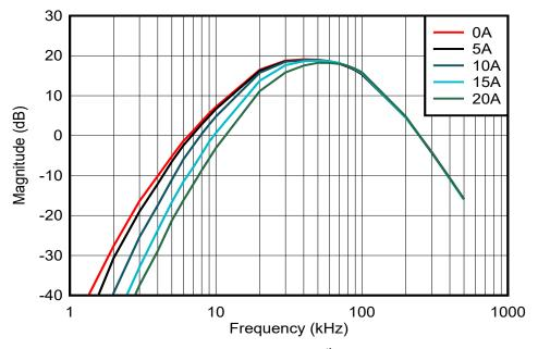
Figure 3-7. Transfer Curve of Analog Signal Chain With 4<sup>th</sup> Order Band-Pass Filter (CH3 and CH4)
