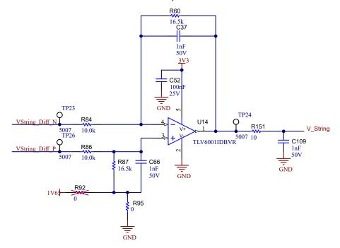
Figure 2-8. Schematics Differential to Single-Ended Conversion
