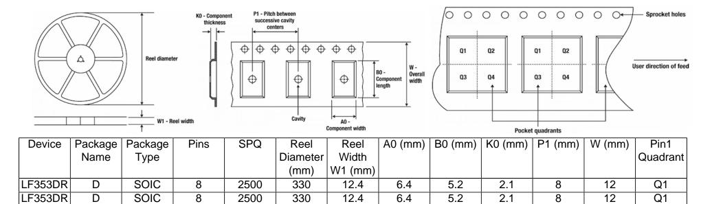
Images above are just a representation of the carrier. Actual carrier may vary. Please reference the dimensions provided in the table.
