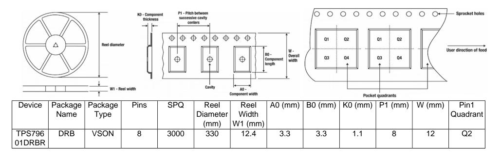
Images above are just a representation of the carrier. Actual carrier may vary. Please reference the dimensions provided in the table.
