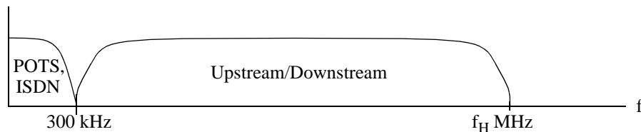
Figure 22. A single band supports both downstream and upstream transmission in TDD systems
