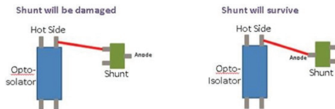
Figure 4: Effects of electric arcs (red line) on shunt references.
