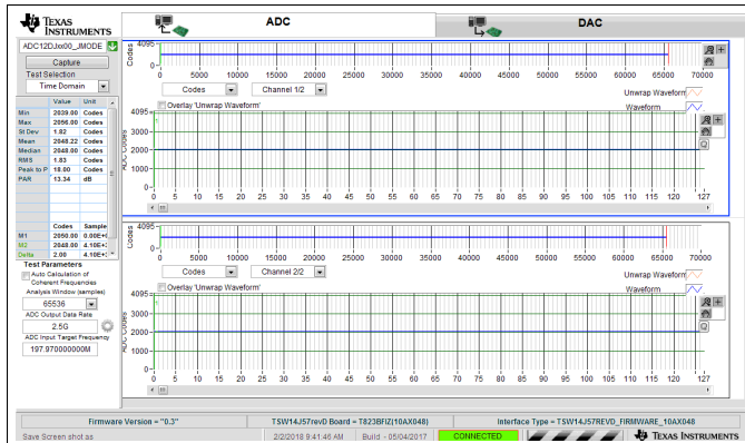
Figure 189. Idle-Channel Noise (No Input) for 2.5-GSPS, Dual-Channel Oscilloscope
