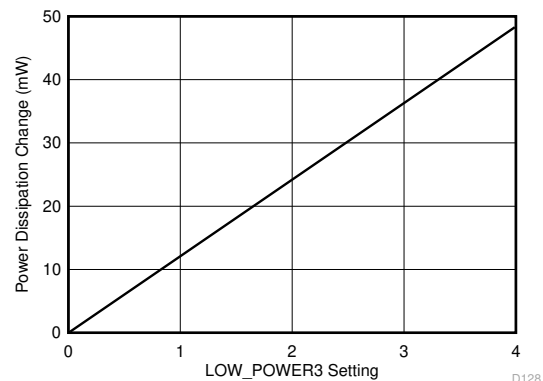
Figure 6-11. Power Dissipation Change vs LOW_POWER3 register setting
