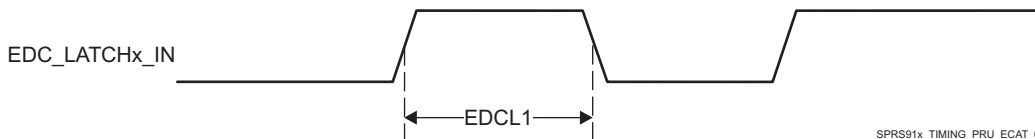
Figure 5-120. PRU-ICSS ECAT LATCHx_IN Timing
