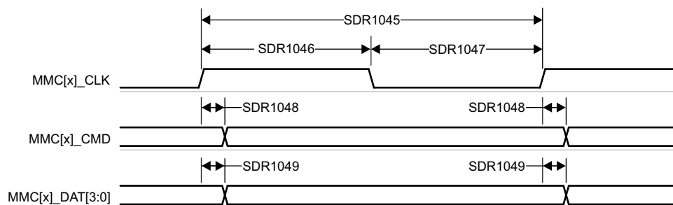
Figure 6-96. MMC1/2 – UHS-I SDR104 – Transmit Mode
