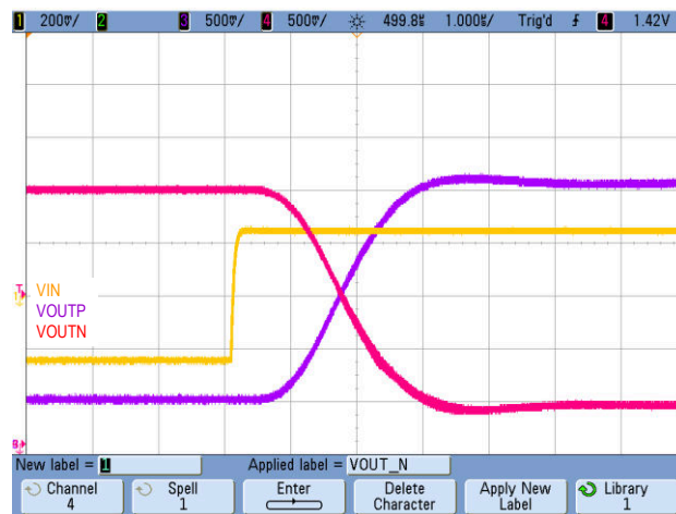
Figure 8-4. Step Response of the AMC1301-Q1
