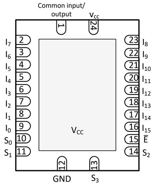
Figure 4-2. RGY Package, 24-Pin QFN (Top View)
