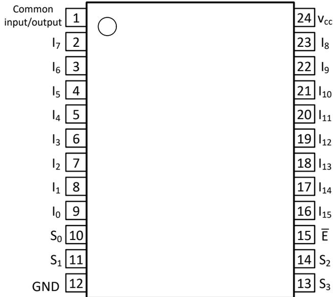
Figure 4-3. PW Package, 24-Pin TSSOP (Top View)
