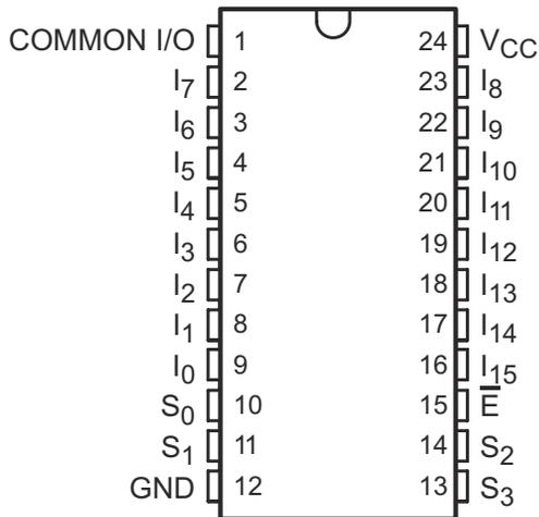
Figure 4-1. DW Package, 24-Pin SOIC (Top View)
