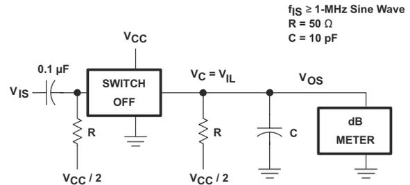
**Figure 14-4. Switch OFF Signal Feedthrough Test Circuit**
