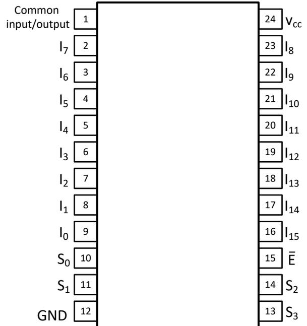
Figure 4-4. DGS Package, 24-Pin VSSOP (Top View)
