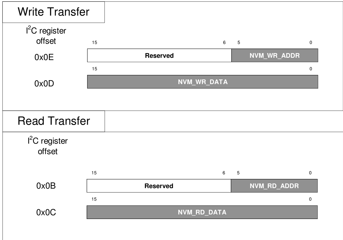
Figure 10-11. EEPROM Direct Access Using I 2 C
