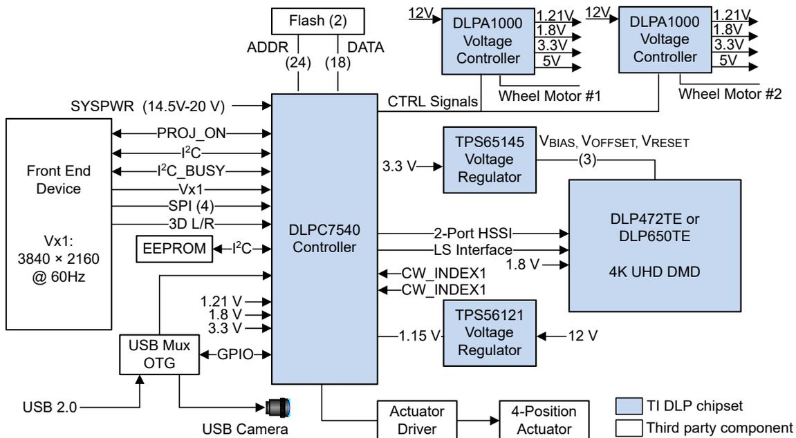
Figure 7-1. Typical 4K UHD Laser Phosphor Application Diagram
