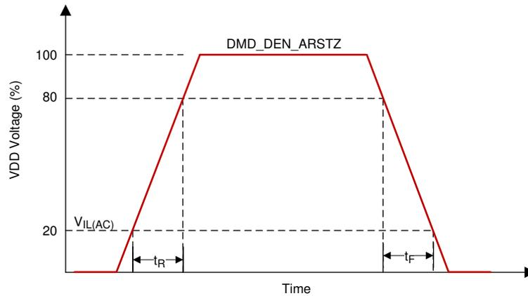
**Figure 5-10. LVCMOS Rise, Fall Time Slew Rate**
