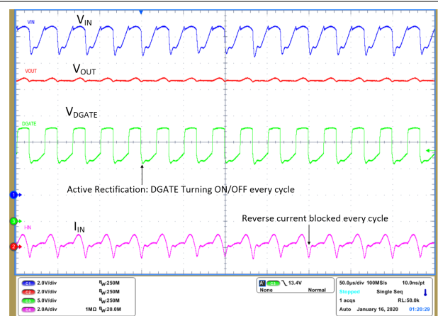
Figure 10-4. AC Super Imposed Test - 2-V Peak-Peak 30 KHz
