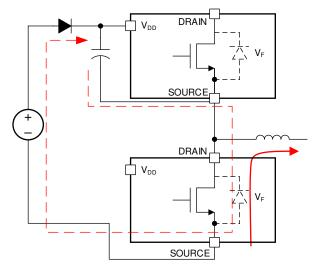
Figure 21. Charging Path for Bootstrap Diode
