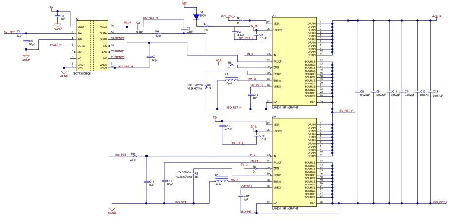
Figure 20. Typical Half-Bridge Application
