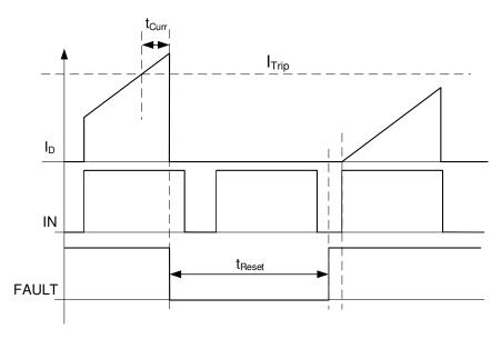
Figure 17. OC Latching and Reset Sequence
