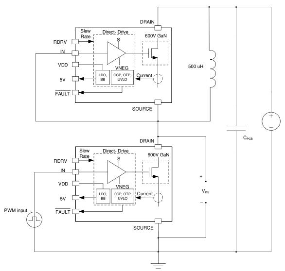
Figure 13. Circuit Used to Determine Switching Parameters
