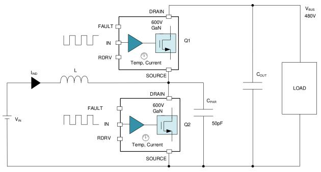
Figure 19. Circuit Used for SOA Curve in Repetitive SOA
