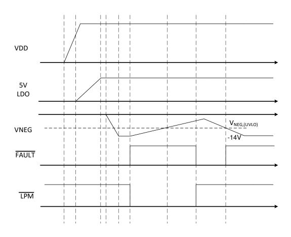
Figure 16. LPM in and out Timing Diagram
