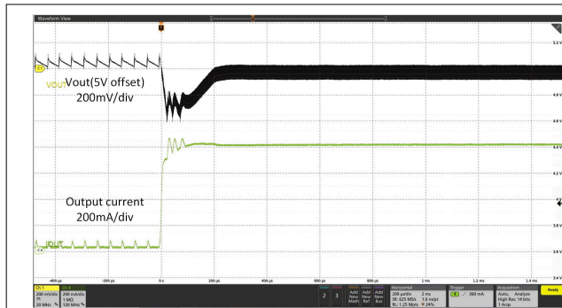
V_{IN} = 3.6V, V_{OUT} = 5V, I_{OUT} = 0A \text{ to } 800mA \text{ Sweep}
